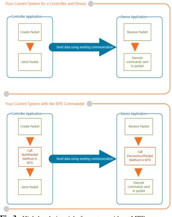
**Fig 3.** High-level pictorial of a system without MTE versus that of a system with MTE.
